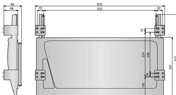
**2 COULISSE AVEC SUPPORT POUR FIXATION SOUS PLATEAU ET BUTÉES D'ARRÊT**
